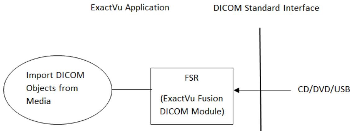
Figure 2: DICOM File-Set Reader Flow Diagram
